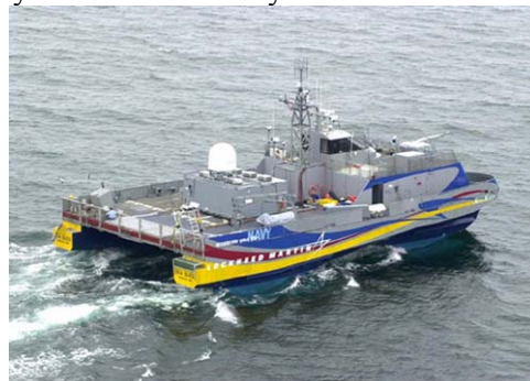
Figure 5: High-speed SWATH type vessel SEA SLICE
